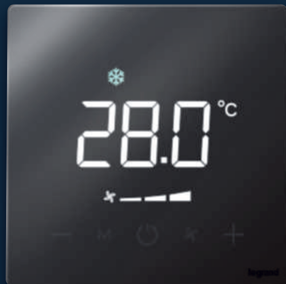
Room temperature control unit
